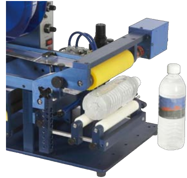
450 Table Top System with Round Product Applicator Module.
