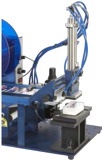
450 Table Top System with Tamp Module.
